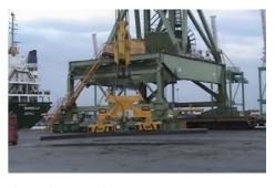
by the slab. Magnet system can be operated from a safe distance using radio control or from the crane operator cabin. No need for slings or clamps.
